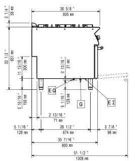
Electrical inlet (power) Gas connection
